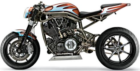
absent, however, is any device that might actually absorb shock. Walk around the bike and you discover that DesJardins has ingeniously mounted the rear shock on the left side, tucked in against the engine and extending the visual line of the subframe. Side holstering the shock also contributed to the mission of shortening the Hellion's wheelbase to a crisp 57 inches.
